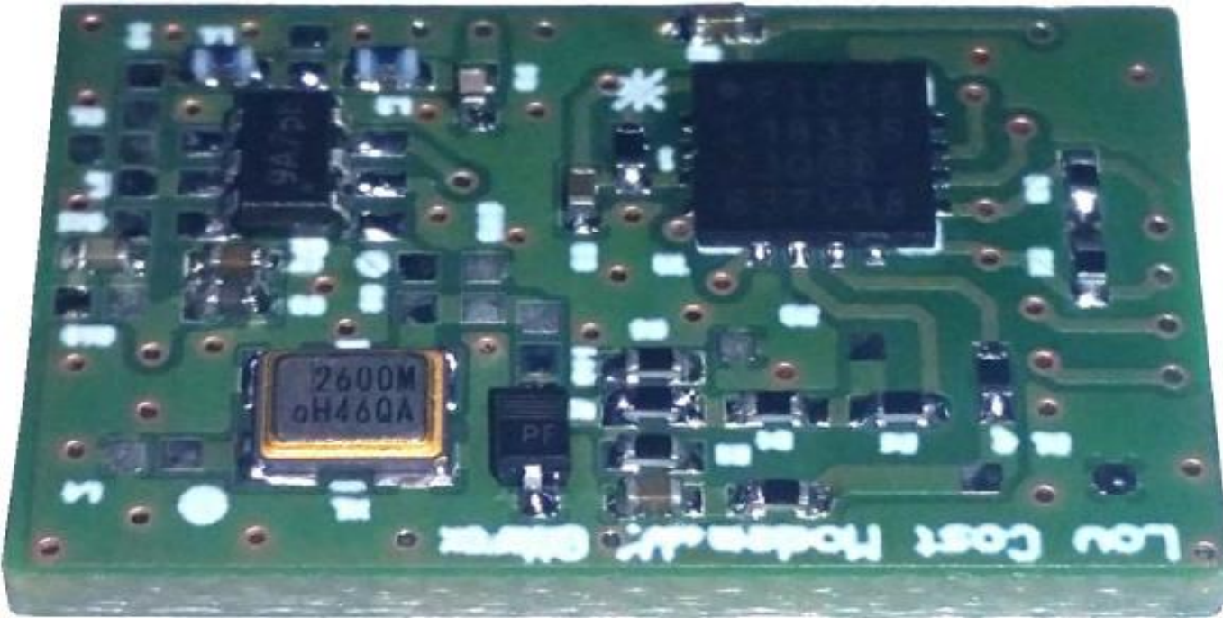
8bit \mu C + FM modulated RF oscillator
