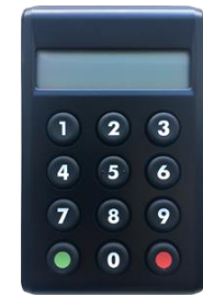
Audio code reader with large display and audio output for visually impaired people
